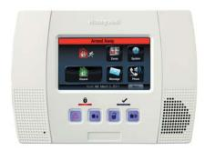
Part of Honeywell's family of self-contained wireless controls, ADT's dynamic L5000ADT has a bright, full-color touchscreen that simplifies security system operation. Whether arming or disarming the system, bypassing zones or leaving messages or reminders for family members, the graphics and intuitive, menu-driven prompts make operation crystal clear—reducing end user training time and false alarms.
